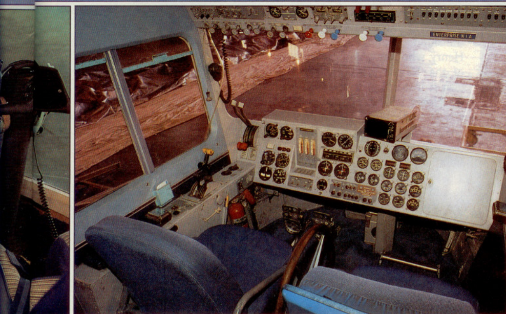
The Spirit of Akron's cockpit (left) is state of the art with electronic instruments and flight control system. The Enterprise (above) is steered with a wooden ship's wheel.
