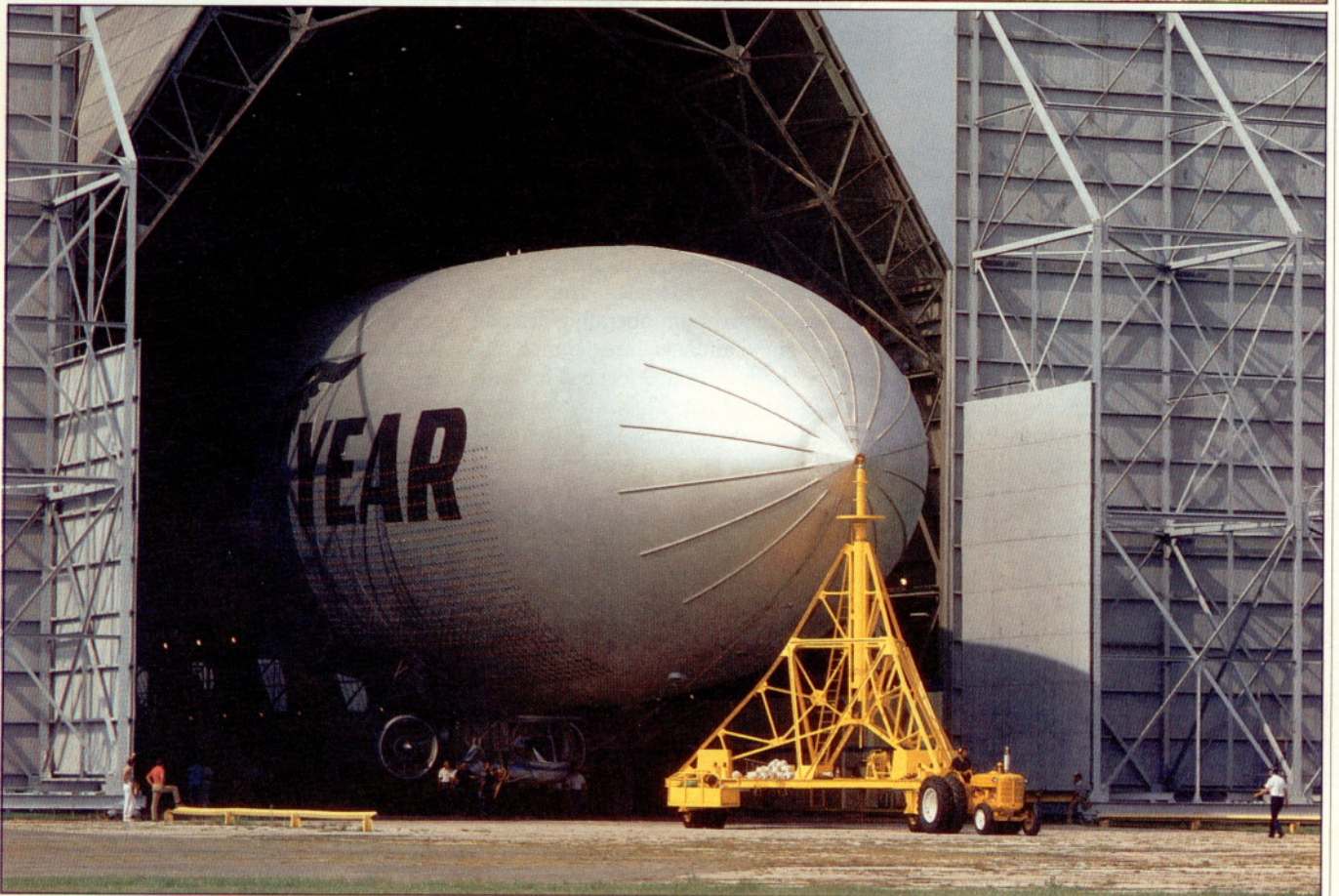
Helium allows a blimp to float free of the earth. A robust ground crew is essential to bringing it back. A mobile docking mast gently tucks the Akron back into its berth in the Wingfoot Lake airdock.
